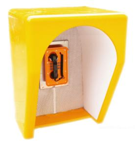
general-purpose resin material to BS476 Class 1 fire regulation, the RF-13 is extremely robust and weatherproof. Inside the hood's outer shell is a perforated polypropylene lining that houses 50mm non-hygroscopic acoustic insulation.
